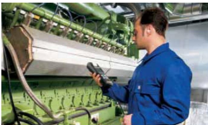
**testo 350 XL: Portable measurements on motors (O<sub>2</sub>, CO, NO, NO<sub>2</sub>)**
