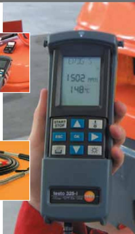
Tuning motors with the CO<sub>high</sub> [O<sub>2</sub>] analyser
