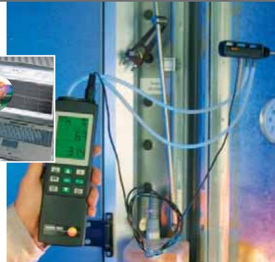
Pitot tube measurement in a flue gas duct
