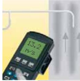
Built-in flow and mass flow measurement (optional)
