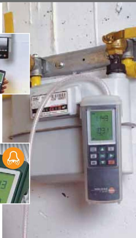
Fuel pressure measurement on stationary gas motors
