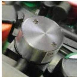
Infrared (NDIR) measurement module for direct CO<sub>2</sub> measurement
