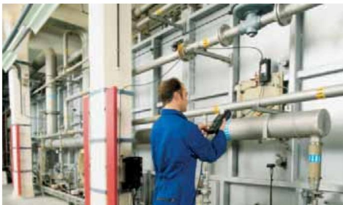
**testo 350 M: Set for fast emission monitoring on industrial burners (O<sub>2</sub>, CO, NO, SO<sub>2</sub>)**
