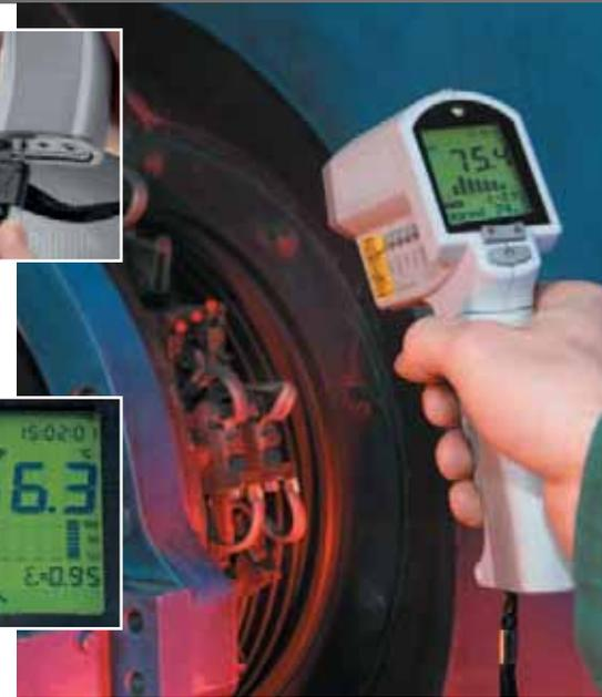
Spot measurements on a gas turbine using testo 860-T2
