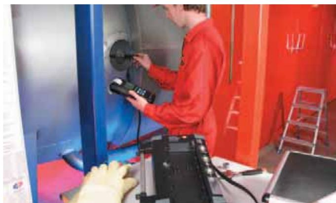
**testo 350 XL: Portable measurements on turbines (O<sub>2</sub>, CO<sub>low</sub>, NO<sub>low</sub>, NO<sub>2</sub>)**
