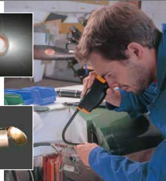
Accurate inspection of welded joints e.g. in hollow spaces
