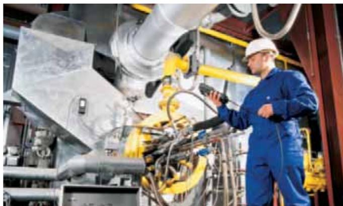
**testo 350 XL: Standard set for measurements on process systems (O<sub>2</sub>, CO, NO, NO<sub>2</sub>)**
