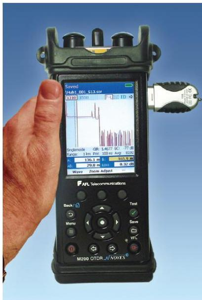
The Noyes M200 from Fujikura Europe offers unmatched OTDR capabilities in a handheld package weighing less than 1 kg (2 lb). Multimode, Single-mode, and 'Quad' wavelength models are offered. With short dead zone and intermediate range specifications, the M200 is ideal for Tier 2 testing of premises (building and campus) networks or certification and troubleshooting of FTTX PON networks. And its bright, transfective display makes it suitable for both indoor and outdoor operation.
