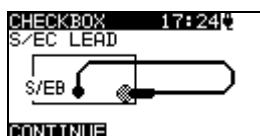
Figure 1.16: S/EB test lead check starting screen
