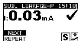
Figure 1.59: Substitute leakage - P result screen
