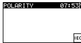
Figure 1.60: Polarity test starting screen
