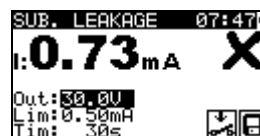
Figure 1.36: Example of substitute leakage current measurement results
