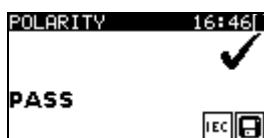
Figure 1.42: Examples of polarity test result
