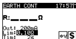
Figure 1.50: Earth continuity starting screen
