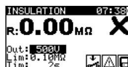
Figure 1.30: Examples of Insulation resistance measurement results
