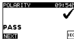
Figure 1.61: Polarity test result screen
