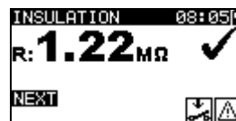
Figure 1.53: Insulation result screen
