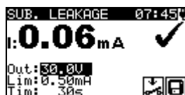
Figure 1.36: Example of substitute leakage current measurement results
