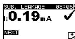
Figure 1.55: Substitute leakage result screen
