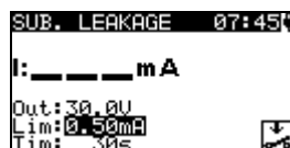
Figure 1.34: Substitute leakage menu
