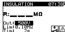
Figure 1.52: Insulation resistance starting screen
