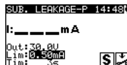
Figure 1.58: Substitute leakage - P starting screen
