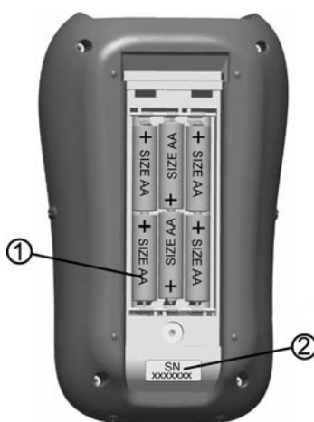
Figure 1.4: Battery compartment
