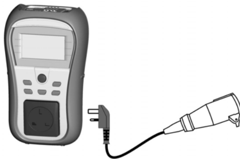
Figure 1.78: Connecting 110 V adapter to the instrument
