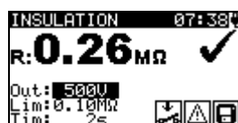
Figure 1.30: Examples of Insulation resistance measurement results
