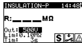
Figure 1.56: Insulation resistance - P starting screen
