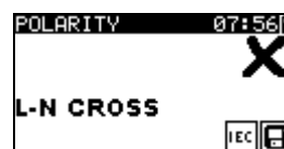
Figure 1.42: Examples of polarity test result
