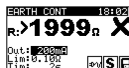
Figure 1.27: Examples of Earth continuity resistance measurement results
