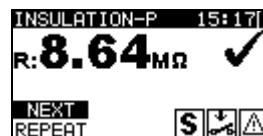
Figure 1.57: Insulation resistance - P result screen
