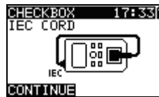
Figure 1.17: IEC test cord check starting screen
